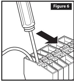
Remove wires from the block by inserting a small flat tip screwdriver into the top slot. Push tip all the way down and push forward. Remove wire.
