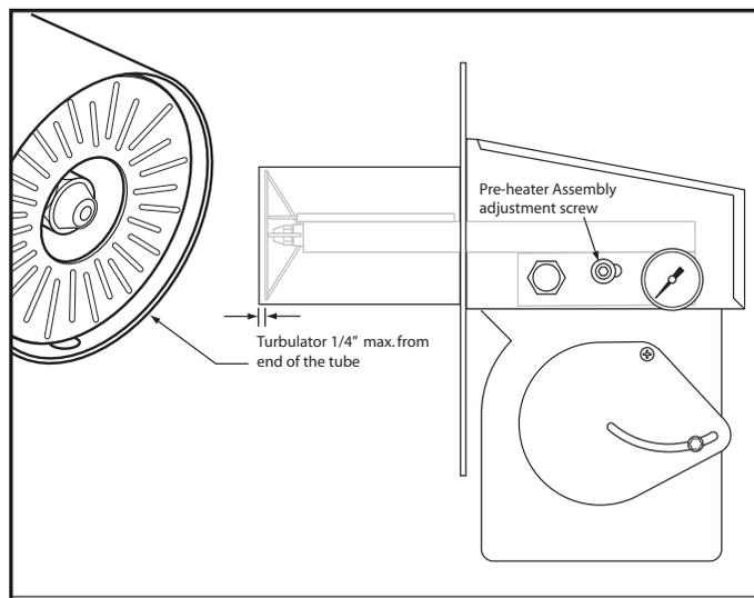
**Air Pre-Heater Diaphragm Breakdown**
